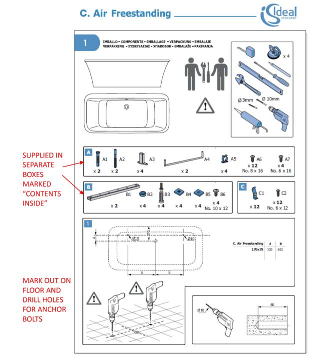
POSITION LEG BEAMS B1 TO THESE DIMENSIONS AND SECURE TO THE BATH 2
