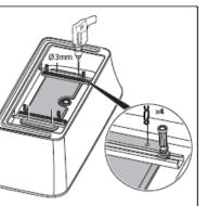
MARK OUT AND PRE DRILL HOLES FOR BEAM C CLIP A5
